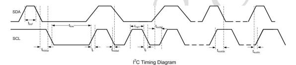
Figure 14. I<sup>2</sup>C Timing Diagram
