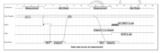
Figure 11 Data Read Sequence at Measurement
