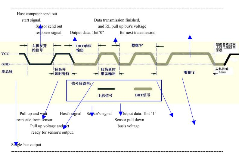
2) Step 1: MCU send out start signal to DHT22
