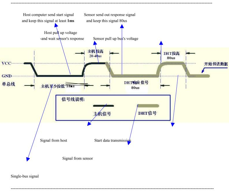
Step 2: DHT22 send response signal to MCU
